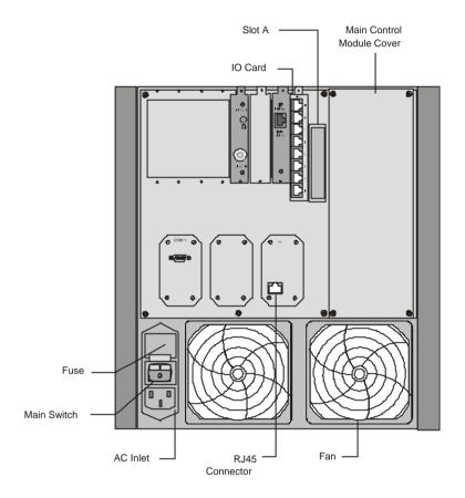
Figure 2-6: MGC-50 Rear Panel with External Connector
